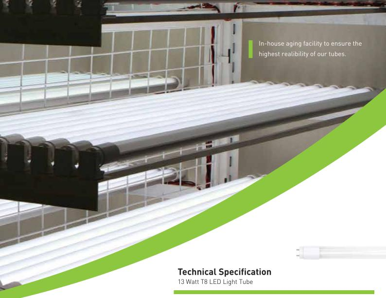
Everlit is one of the first in the world to produce a 13 Watt T8 LED tube with 1800 lumens output. Our T8 tube is able to achieve a high efficacy of light output by utilizing Nichia LED components. With an aluminium heatsink and PCB design we are able to dissipate heat effectively and have a sturdeier construction.
